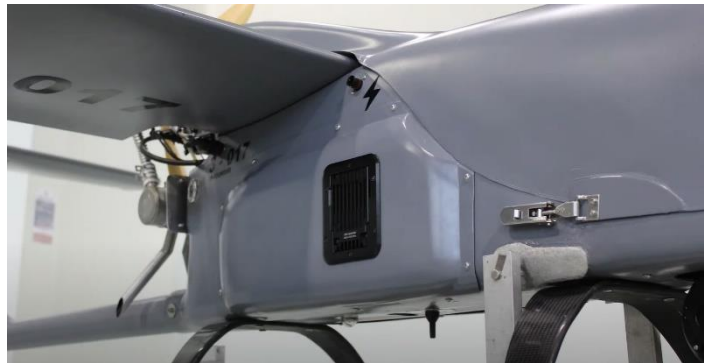
[Caption] Embedded Module aboard the UAV
